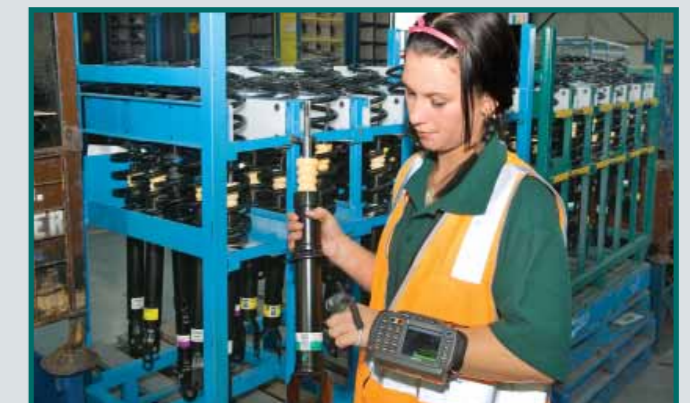
A sequencing operator wears the latest arm worn Mobile Data Terminal with finger RF scanner to provide freedom of movement for picking and scanning larger parts.
